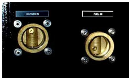
1-1/2" NPT Inlet Connections for Oxygen and Fuel
