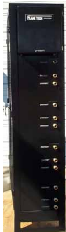
3/4" NPT outlet connections grouped by torch
